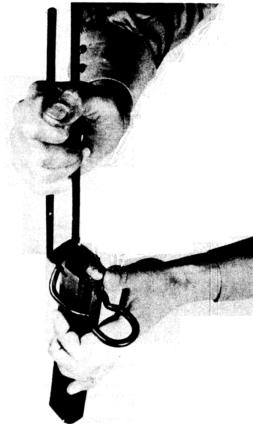
Figure 28. Use of the stock as a hand loader.
